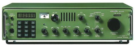
Main Receiver R1120 10 kHz - 30 MHz SSB Telephony - Telegraphy - Telex
